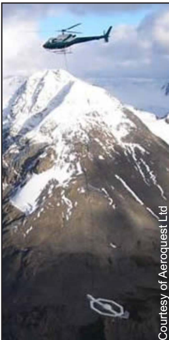
Figure 2: Aeroquest Ltd's helicopter-borne TEM System, AeroTEM.
