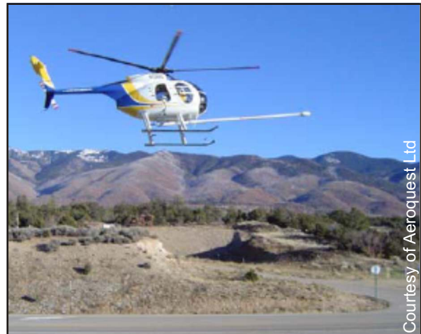
Figure 1: Aeroquest Ltd’s helicopter-mounted ‘stinger’ magnetometer.
