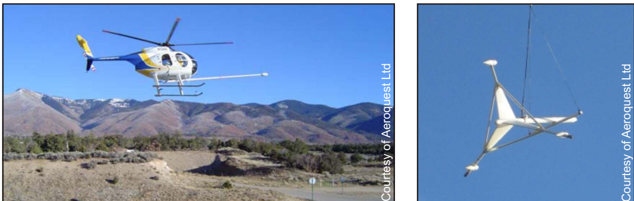
Figure 1: Aeroquest Ltd instruments. Right: stinger (single magnetometer). Left: TAG (triaxial gradiometer).
