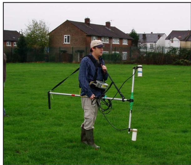
Figure 2: Ground-based magnetic gradiometry survey in progress.
