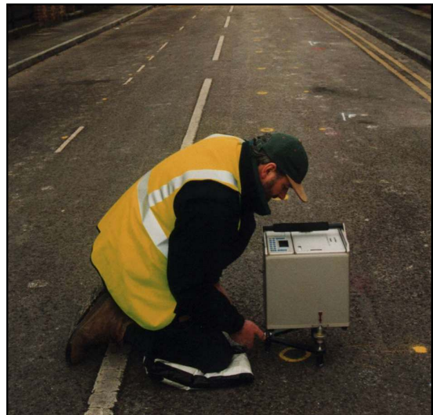
Figure 1: Acquisition of micro-gravity data in a built-up area.
