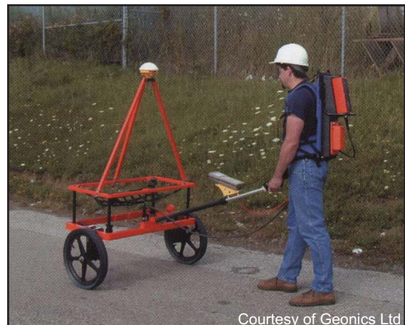
Figure 1: Left: Coil configuration of original EM61 Mk 1 showing orientation of magnetic field relative to target. Right: Geonics EM61 Mk 2 operated in trolley mode. The coincident coils T_x and R_{x1} are located in the lower quadrangle, whilst the upper quadrangle houses R_{x2} . Survey positioning data are acquired using a GPS antenna mounted above the coils.
