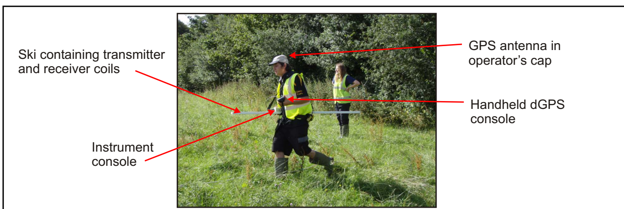
Figure 1: A GEM-2 survey in progress using a vertical dipole/horizontal coil orientation.
