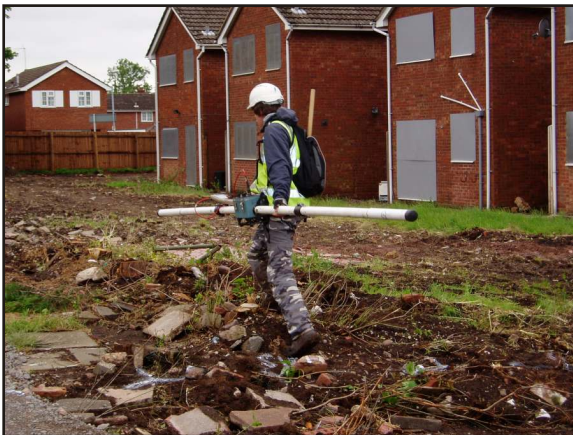
Figure 1: Acquisition of EM31 data on two former industrial sites to map foundations, underground storage tanks, voids, pipes, culverts and possible contamination plumes.
