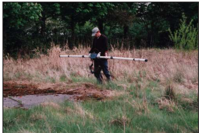
Figure 1: Acquisition of EM31 data.
